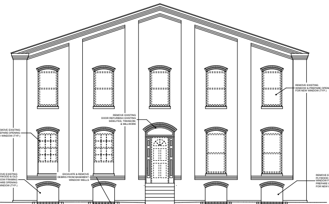
2 FRONT ELEVATION - DEMOLITION SCALE: 1/8" = 1'-0"
