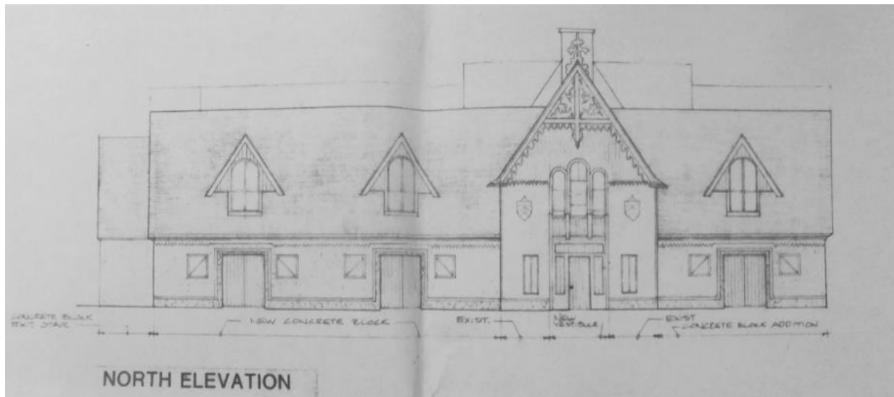
Figure 5: Proposed north elevation, 1980, showing east and west additions.
