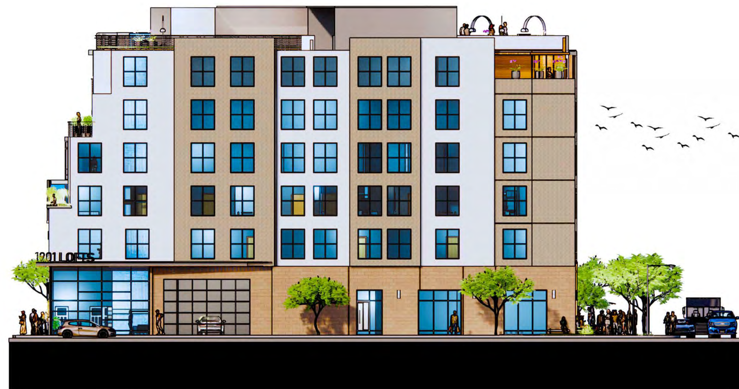
NORTH BUILDING ELEVATION - WEST NORRIS STREET SCALE: 1/8" = 1'-0"
