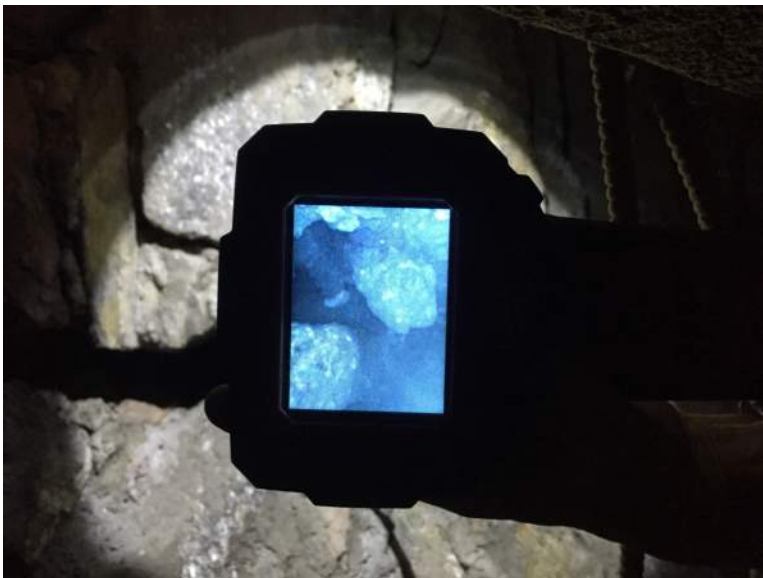
Boroscope readings behind the diagonal infill wall indicates a void originally built. Based on the boroscope readings, the void was filled with dust, remnants of former mortar (damaged through age and freeze/thaw).
