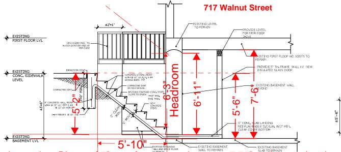
Code requires Risers of 7" max for egress, these are 7.75" and exceed code. Nose of bottom step to lintel has less than 6'-8" headroom required.
