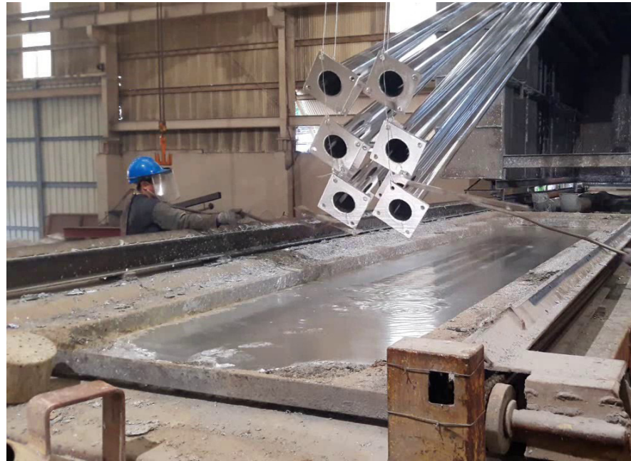
10" Diameter Support Poles - HDG Steel Hot-dip galvanizing is a process of applying a protective zinc coating by dipping product in bath of molten zinc. Galvanizing is a favored method of protective coating due to its low cost, ease of application, and long maintenance-free service life. More detailed information in the Materials Cut Sheets at the end of this presentation. Pg 6
