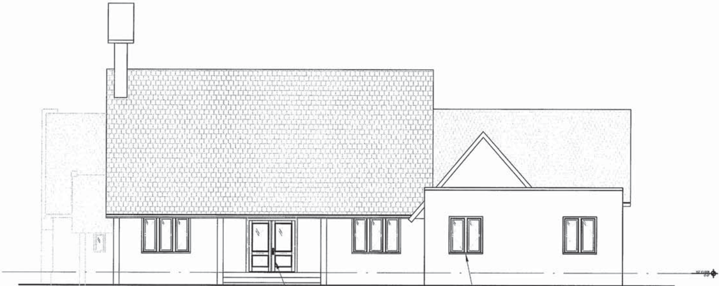
1 ELE-4 EXTERIOR ELEVATION: McMICHAEL SIDE- PROPOSED 1/8" = 1'-0" NEW PATIO DOORS IN EXISTING WINDOW OPENING NEW WOOD WINDOWS, TYP. EXISTING WINDOW MILLWORK TO REMAIN, TYP
