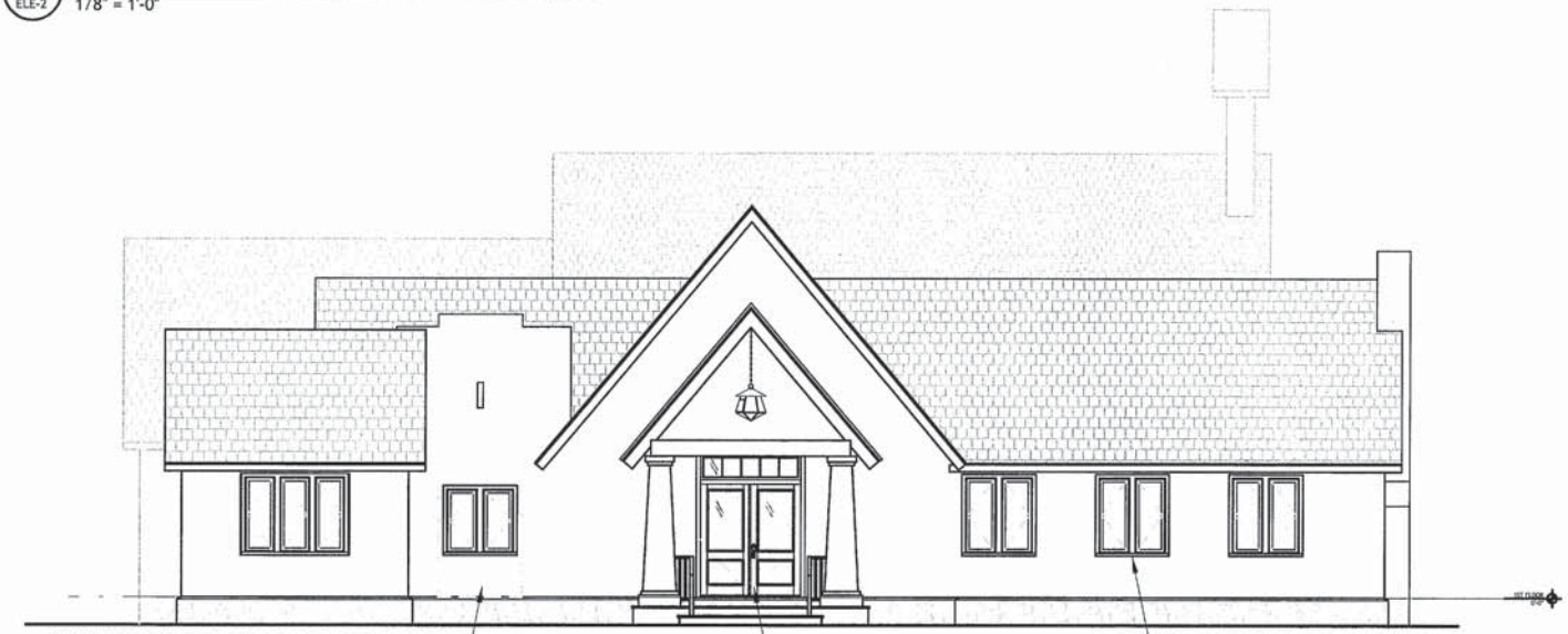
1 ELE-2 EXTERIOR ELEVATION: MIDVALE FRONT- PROPOSED 1/8" = 1'-0" INFILL W/ STUCCO TO MATCH BELOW NEW WINDOW NEW PORCH AND ENTRANCE DOORS AT EXISTING WINDOW LOCATION NEW WOOD CASEMENT WINDOWS, TYP. EXISTING WINDOW MILLWORK TO REMAIN, TYP
