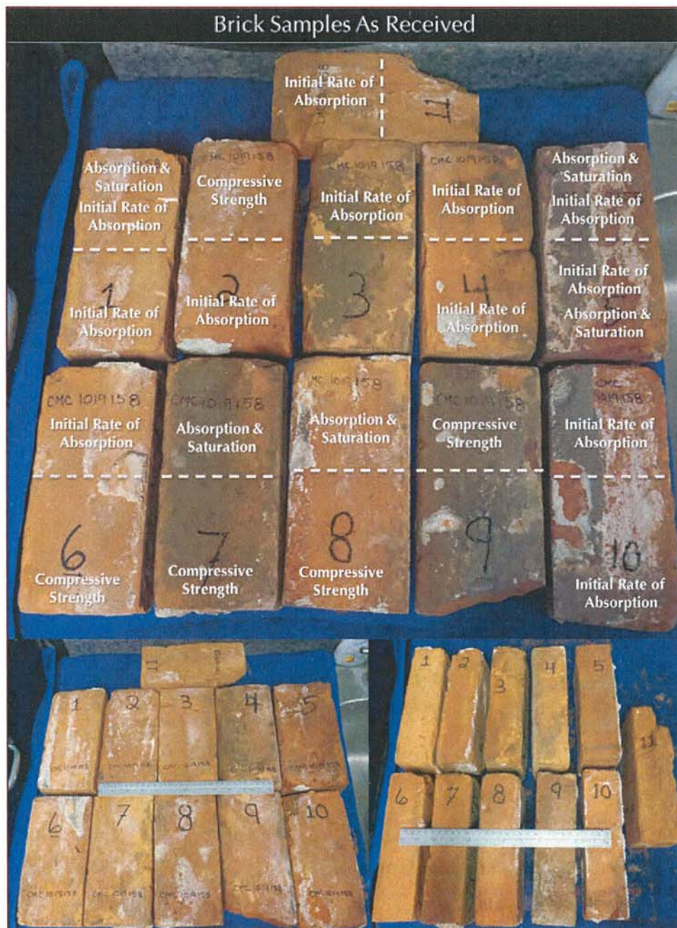
Figure 2: Shown are eleven brick units identified as Nos. 1 through 11. White dashed lines on bricks indicate locations to cut; portions were used for compressive strength testing, and the opposite portions were used for absorption, etc.
