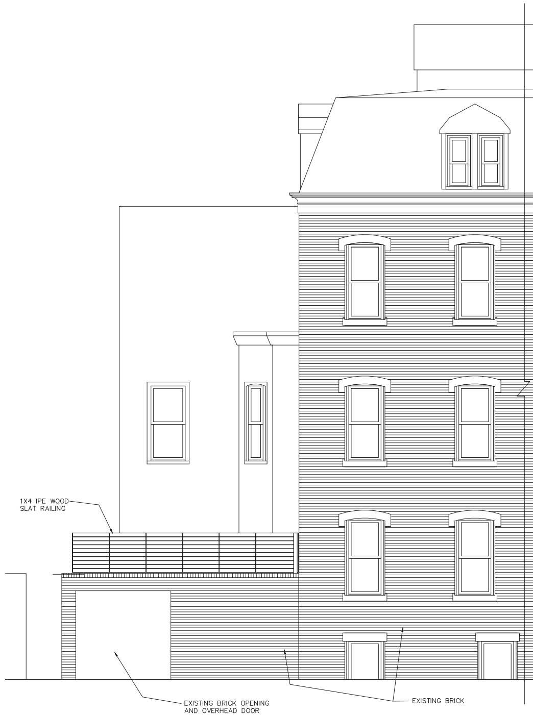
6 PARTIAL EAST EXTERIOR ELEVATION A1.2 SCALE: 3/16" = 1'-0"
