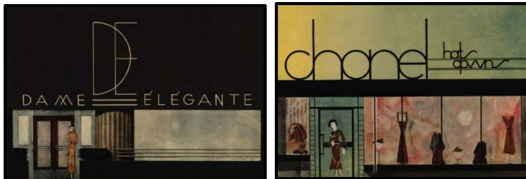
Published in 52 Designs to Modernize Main Street with Glass in 1935, the above designs for “The Apparel Store” are decidedly Art Moderne, using glass panels, open fronts, and distinctive signage to attract the customer. Figure 15. Left: Design No. 652 by Herbert L. Rodde. This design features what was considered “an exceptionally attractive exterior and at the same time...a novel yet not quite practical window.” 14 Figure 16. Right: Design No. 183 by Irwin A. Sugarman. This design features an “abundance of window display,” an “unusual sign arrangement...equally effective day or night,” and “sign lettering and exterior metal trim” known as Aluminum in a “Coloral” Black finish.” 15 Source: Archive.org.
