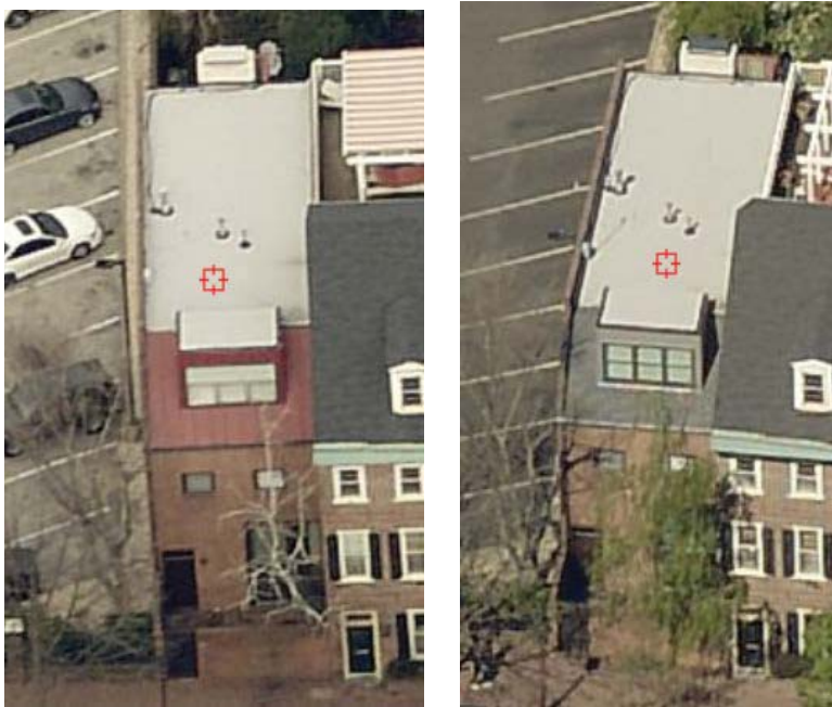
Figure 2: Left, April 2014. Right, May 2015, showing un-approved modifications to the roof and dormer.
