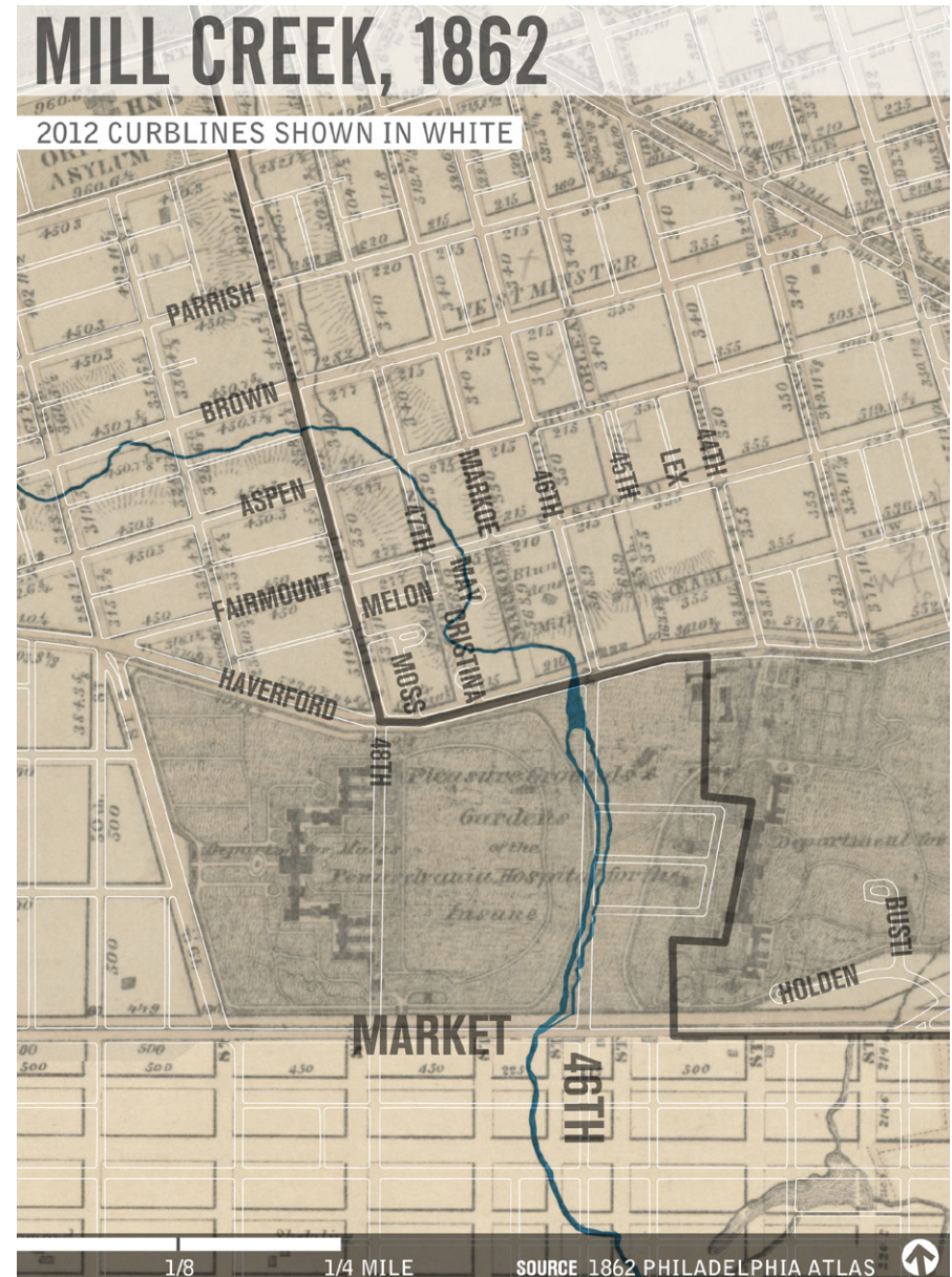
burying mill creek in 1883 [left] eventually led to the collapse of streets and houses built on top of the faulty infrastructure [right].
