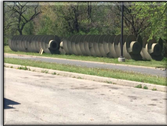
Figure 20: Influent Screw Pump Scheduled to be Replaced
