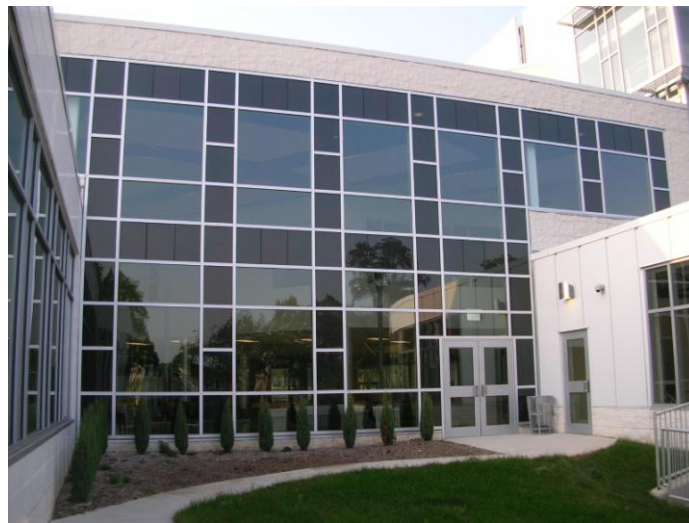
Figure 2-3: BIPV example, PV modules integrated into windows, Microsoft School, Philadelphia
