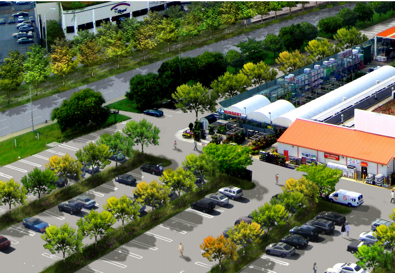
Above: A vegetated swale collects and infiltrates stormwater from an employee parking lot at the Philadelphia International Airport in the Schuylkill Watershed.
