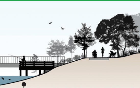
Section through rehabilitated riparian buffer and trail
