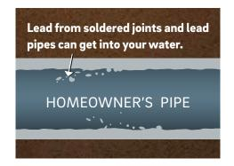
As water stands in your home's plumbing, lead from the soldered joints and old lead pipes can get into your water. Other debris can build up on the aerator, too. It's important to clean faucet aerators and screens to remove any debris from them.
