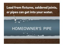
As water stands in your home's plumbing, lead from the soldered joints and old lead pipes can get into your water. Other debris can build up on the aerator, too. It's important to clean faucet aerators and screens to remove any debris from them.
