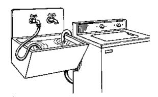
to be cross connections. The direction of flow depends on the pressure differential between the two systems.
